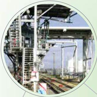
Corrosion and slip-resistant Fibergrate® products including stair treads, handrail, grating, and structural profiles provide access platforms to fuel cars.
