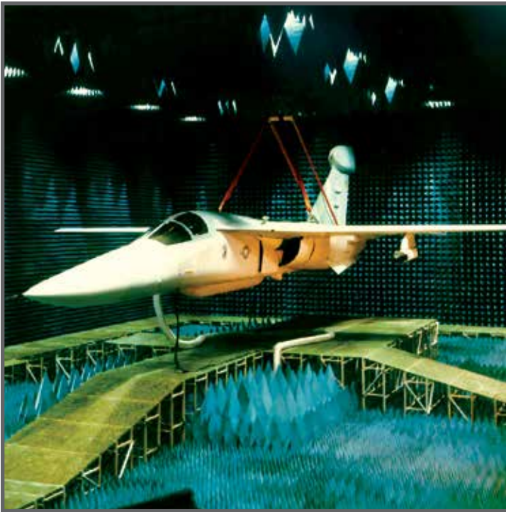
This all FRP (fiberglass reinforced plastic) structure was specifically designed for a General Dynamics anechoic testing chamber. FRP was required because its properties are transparent to the radio and electromagnetic waves used during aircraft testing.
